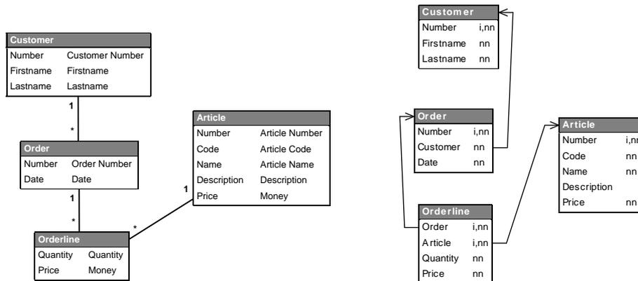
*An example model represented as UML and ERD diagram.*
